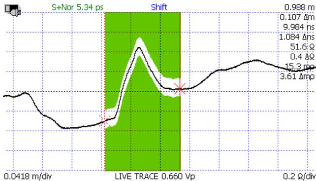
Figure 4.33. A trace that passes the mask test.
