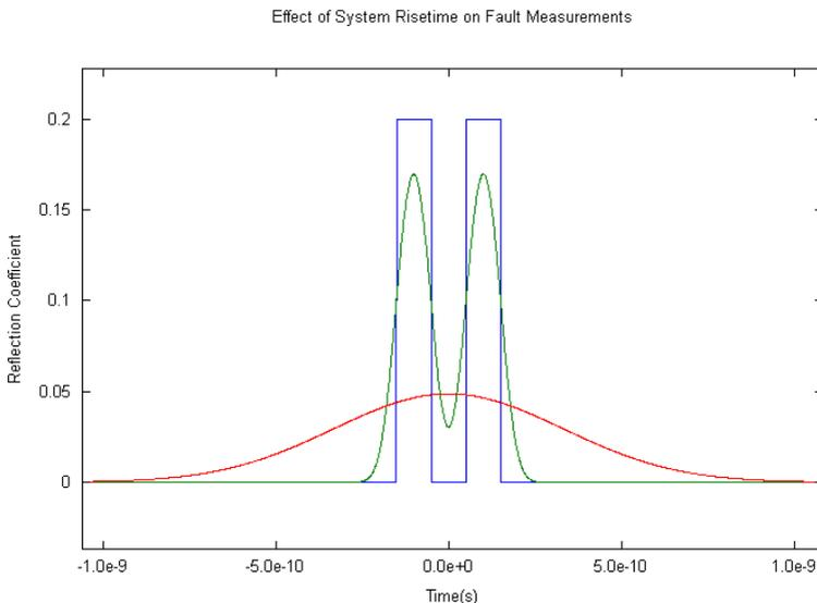
**Figure 7.9.** Simulated comparison of a 90 ps rise time TDR (green) and an 800 ps TDR (red) with respect to the ability to depict two 1 cm long, 75 ohm faults spaced 1 cm apart on a 50 ohm cable. Notice how the faster TDR (90 ps) resolves each fault individually. The blue lines represent a theoretically perfect response.
