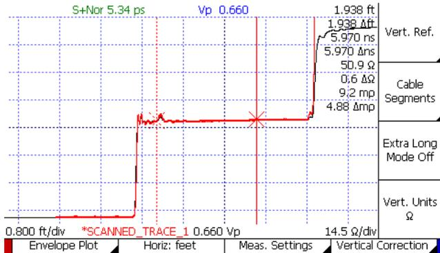
**Figure 3.11.** TDR trace with impedance vertical units (red, top) demonstrating vertical scale in ohms and emphasis of the open fault at the end of the cable. The black trace uses reflection coefficient (millirho) as its vertical units.
