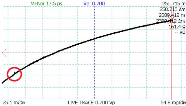
**Figure 3.10.** A small fault in a long cable. This fault (red circle) in an approximately 800 ft. (250 m) cable is from a 3 cm barrel connector (0.01% of cable length). The sampling of the Normal sample resolution setting ensures that the cable fault is displayed at this large horizontal scale (~50 cm/pixel).
