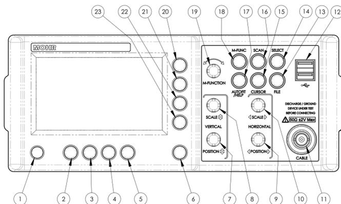
Figure 3.2. Diagram of the CT100B front panel.
