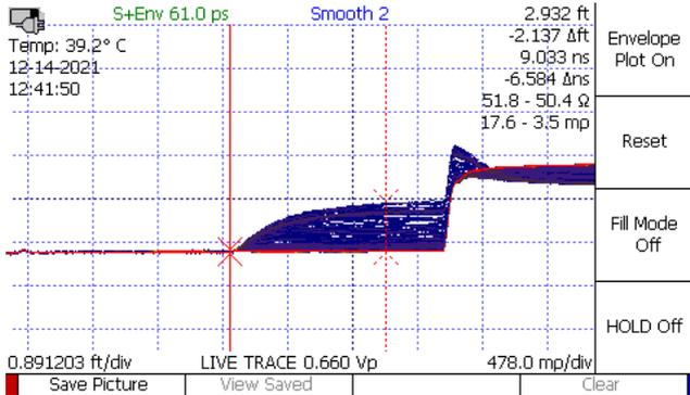
**Figure 4.36.** Envelope Plot with Frequency Density display.
