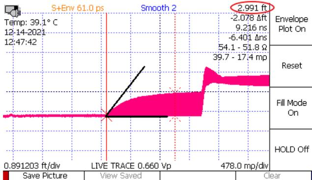
**Figure 4.35.** Envelope Plot with Fill Mode, with the active cursor positioned at the fault location (red circle). Note that the black lines shown here to emphasize the “virtual arrow” do not actually appear on the instrument screen.
