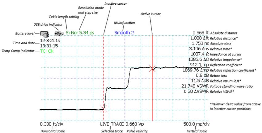
**Figure 3.9.** Screenshot showing typical features of the CT100B.
