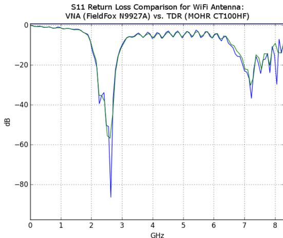
**Figure 7.10.** Comparison of  $S_{11}$  return loss of a 2.4 GHz WiFi patch antenna measured using a handheld VNA (Agilent® FieldFox N9927A, green) and TDR (CT100HF, blue), showing good agreement from DC to ~8.3 GHz. Note bandpass in the 2.4 GHz region.
