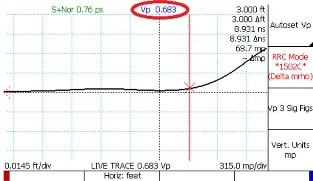
Figure 4.7. Final Vp of the cable.
