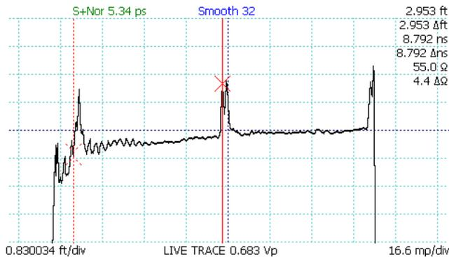
**Figure 4.10.** Vertical scale used to emphasize cable fault.
