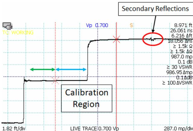
**Figure 5.8.** Using a phase stable cable to improve S-parameter measurements on short microwave cables. Use the phase stable cable (green arrow) and position the rightmost cursor to the left of the secondary reflections (red circle) occurring after the open or short at the end of cable under test (blue arrow) so that they are excluded.
